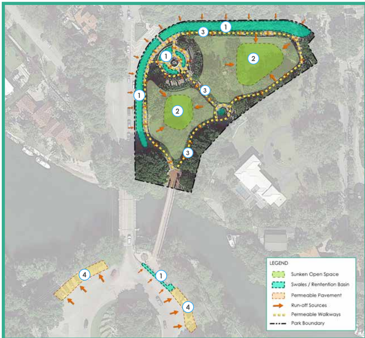
Figure 4-3: Potential Neighborhood Drainage at Ingraham Park
